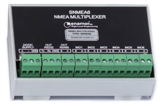
SNMEA6 can even work as splitter and multiplexer at the same time. Arriving protocols are buffered and then retransmitted to allow change of baud rate. Protocol is verified by check sum (if available) and if it doesn't match - rejected. The sum of baud rate of every input must be less then baud rate of output. In SNMEA6 multiplexer all ports are designed to half duplex communication (only one way – TX or RX in one time), what causes that inputs/outputs RS422 also are described like RS485.
