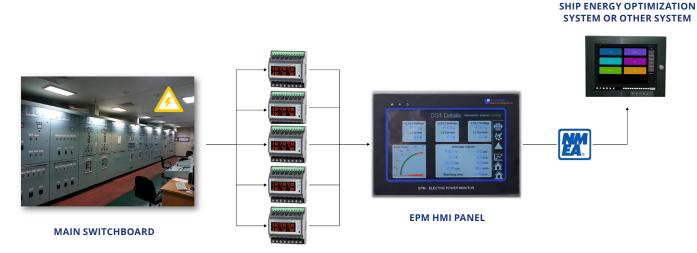
3 PHASE CURRENT AND VOLTAGE TRANSDUCERS UP TO 5 DIESEL GENERATORS
